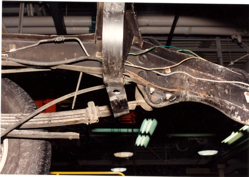
32. Close-up view of the rear tank strap and left frame rail from the right side of the vehicle
